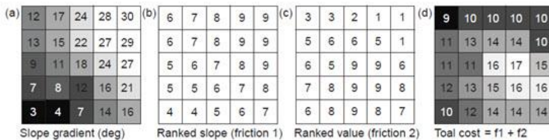
Fig. 1.8 (a) Slope gradient in degrees; (b) ranked (reclassified) slope gradient constituting the first cost or friction input; (c) ranked land value (produced from a separate input land-use raster) representing the second cost or friction input; and (d) total cost raster produced by aggregation of the input friction rasters (f1 and f2). This total cost raster could then be used within a cost-weighted distance analysis exercise.
